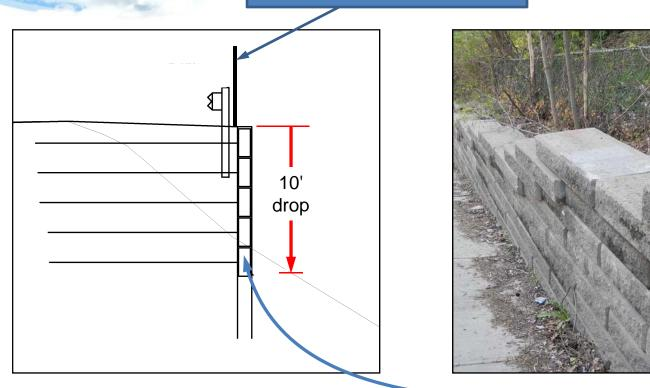
Shoulder widening would create a 10'-high retaining wall, more than 90' long
