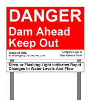
Figure B.3: Primary sign with siren sign mounted below and optional pictograph panel on the left
