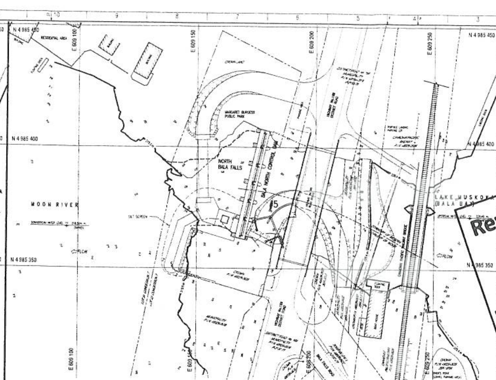
STAGE #5 DEFLECTOR WALL AND INTERMEDIATE COFFERDAM CONSTRUCTION
